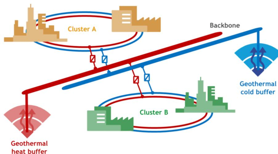
Note: In reality the Heerlen Minewater energy grid is more complex and also has four clusters rather than two. The water from the clusters is separated by heat exchangers from the water in the backbone.
