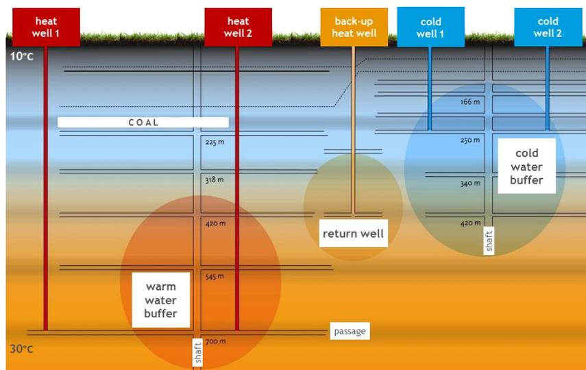
NB: In the latest Minewater concept the return well has been taken off-line, now serving only as a back-up.
