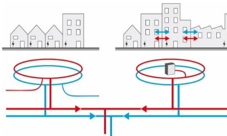
In this phase the two concepts are integrated around a shared backbone, creating an optimized, sustainable energy concept in which the subsurface can be used indefinitely as a heat source and buffer, and supply and demand of heat and cold are optimally balanced. The backbone provides excellent scope for further system upscaling.
