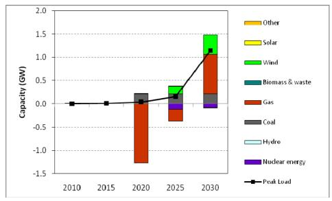
Figure 70 Differences in the UK-Ireland Block capacity mix forecast between Scenario 2 and the Reference Case
