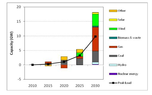
Figure 17 Net changes in the EU capacity mix forecast between Scenario 2 and the Reference Case
