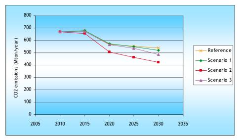
NB. Emissions from petrol and diesel are well-to-wheel, emissions from electricity include power production emissions only (not emissions due to, e.g. coal mining or gas production).
