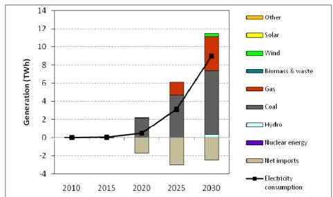
Figure 77 Differences in the South-East Block generation mix forecast between Scenario 3 and the Reference Case
