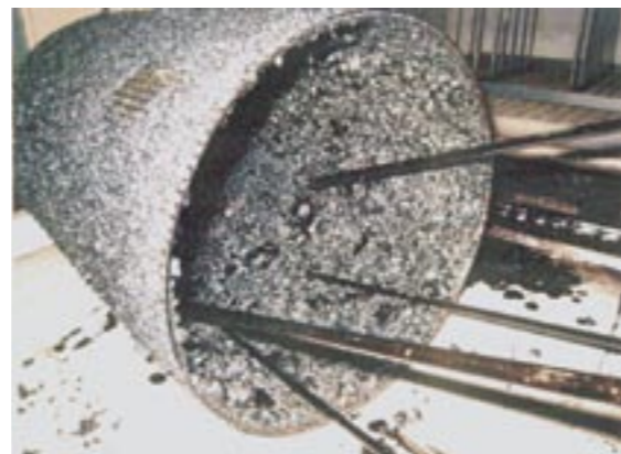
Figure 5 Damage to a ship's engine due to polystyrene deposits in the filter system
