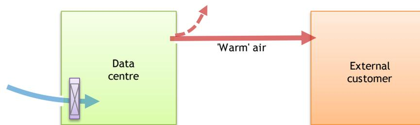
Figure 17 Heat flows of Subvariant 4b. In wintertime the data centre is cooled with free cooling via the atmosphere and the cold reservoir is regenerated
