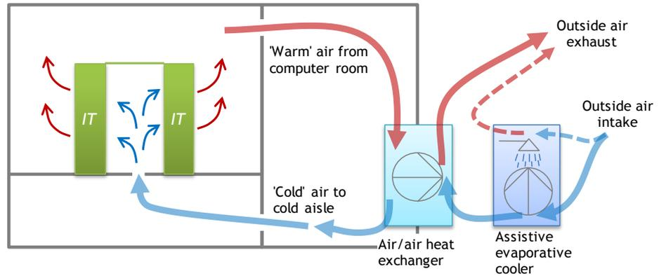
Figure 14 Heat flows and cooling layout of Subvariant 2b with assistive compression cooling in the inside air section
