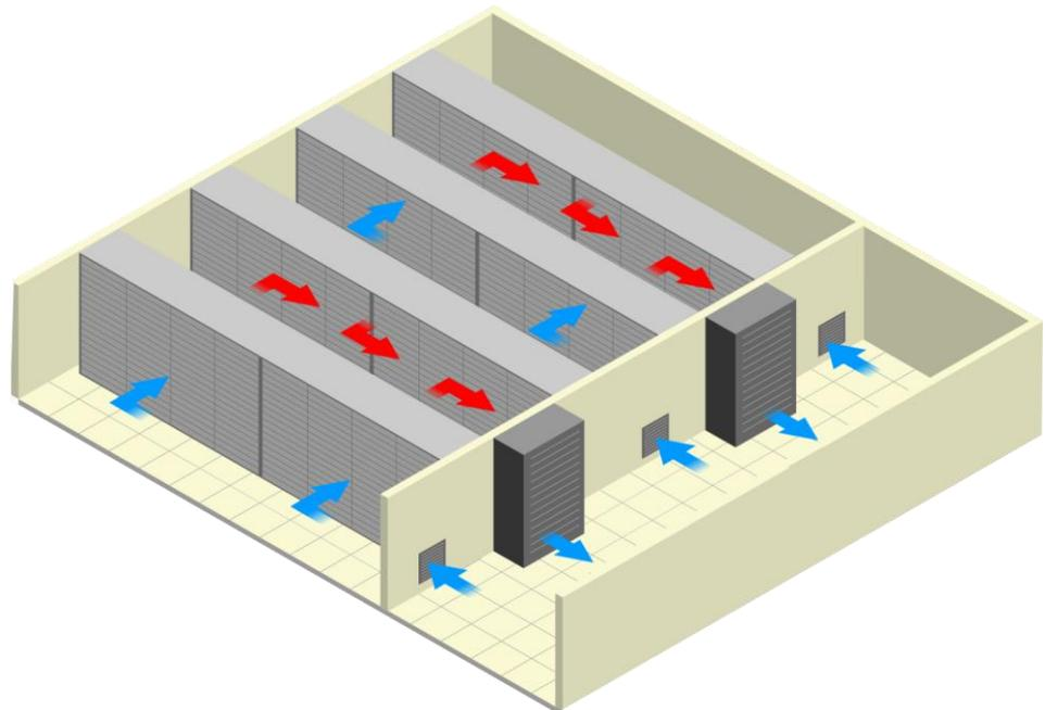
Figure 6 Example of full separation of cold and heat air streams in data centre. The photo shows a cold alley, with influx of cold air via the bottom
