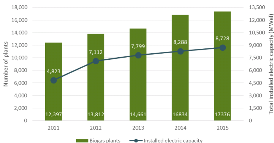
Figure 3 Development of the number of biogas plants and installed electric capacities in the EU
