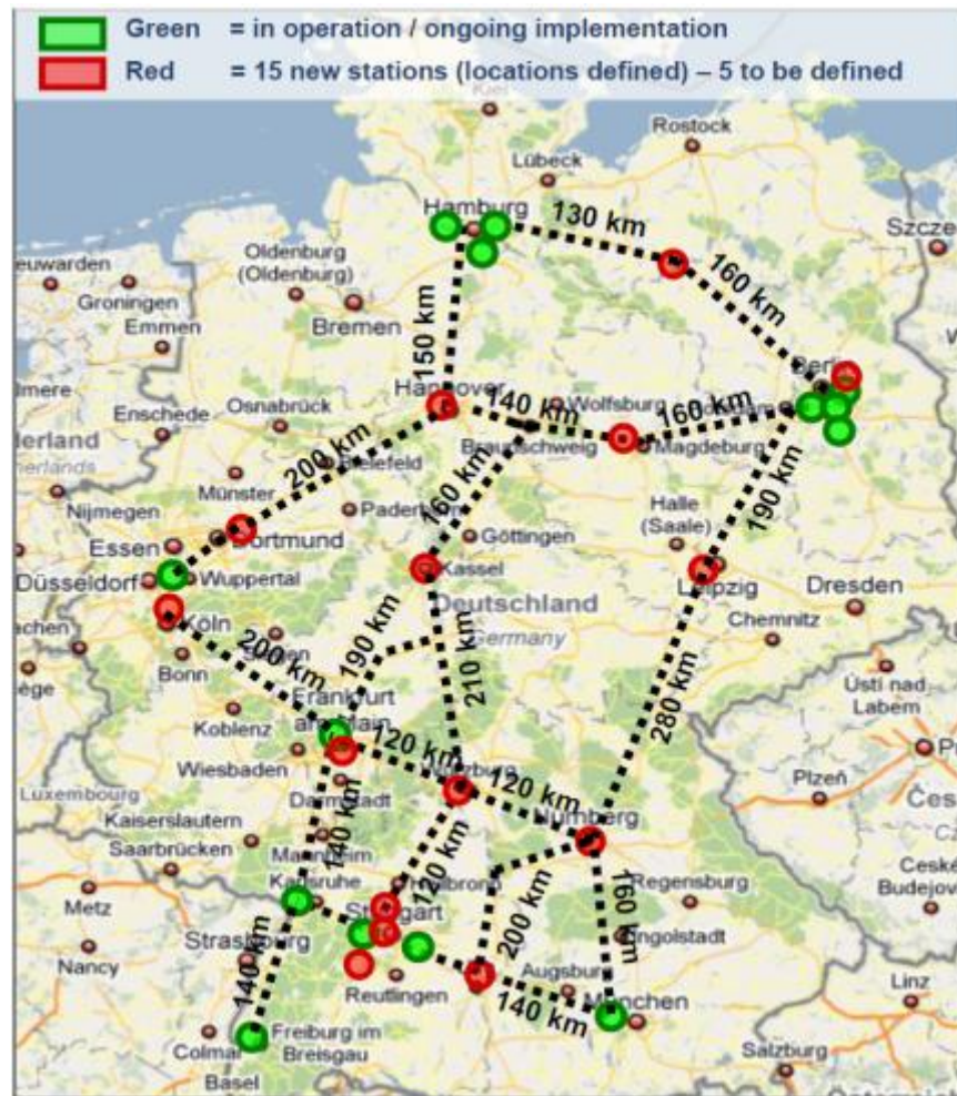
Figure 24 H 2 infrastructure development plans for Germany as laid out by the 'H 2 Mobility' initiative
