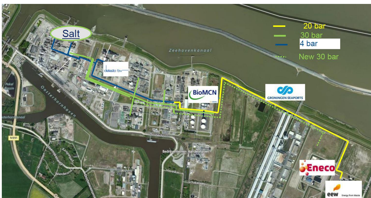
Figure 2-12 Example of process heat distribution grid with third party access in Delfzijl 13 , 14 .
