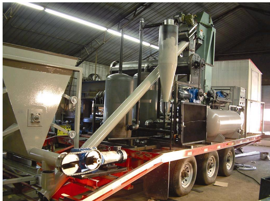
Figure 33 Impression of current catalytic pyrolysis plant
