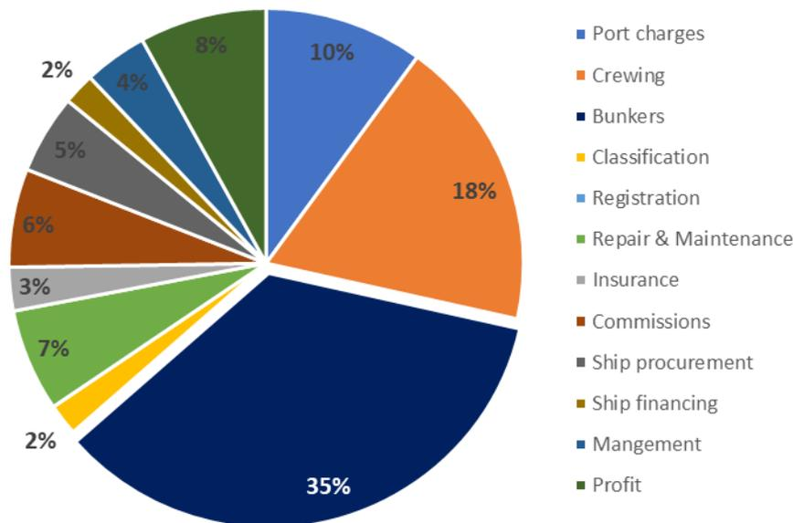
Figure 5.10 Freight rate components of a small tanker (10.000 dwt) with 20 years of economic life
