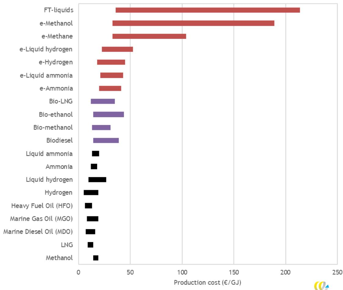
Figure 3.4 Current production cost of sustainable alternative fuels vs. fossil fuels for maritime ships (black: fossil fuels of fossil-fuel based; green: biofuels; blue: e-fuels with renewable electricity)
