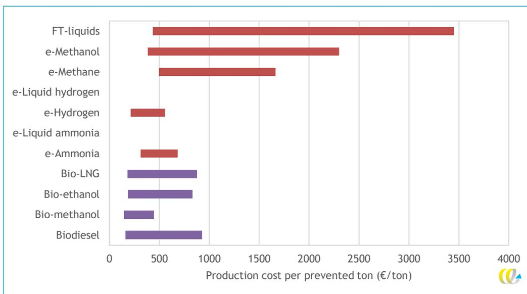
Figure 3.10 Current production cost per ton of CO<sub>2</sub> reduction for alternative marine fuels
