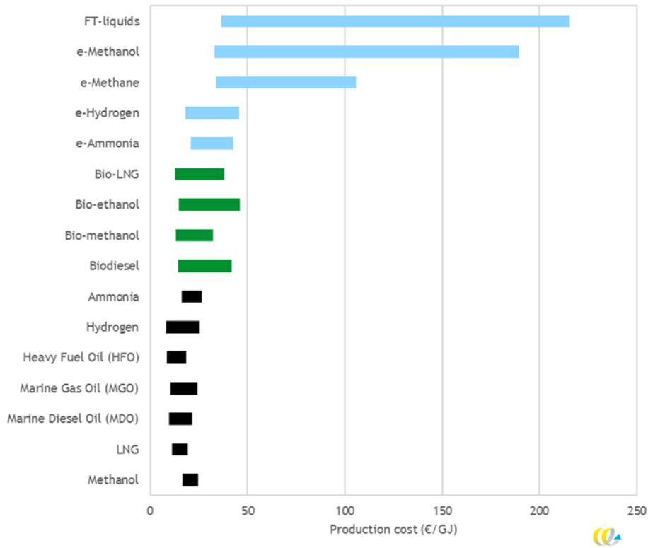
Figure 3.11 Carbon-adjusted production cost of marine fuels, assuming a carbon price of 30 to 60 €/ton
