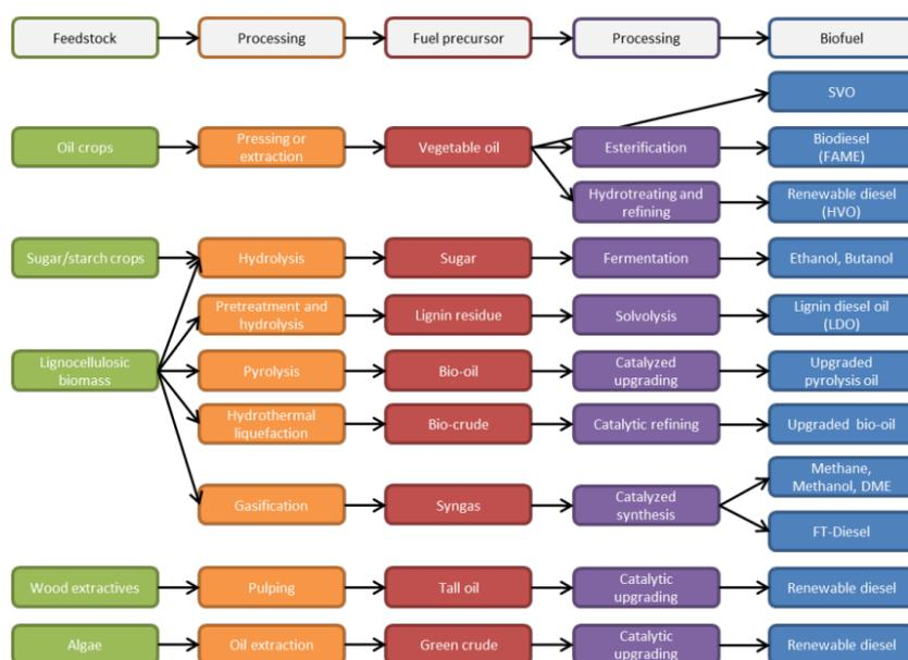
Figure 3.3 Overview of different feedstock conversion routes to marine biofuels including both conventional and advance biofuels.
