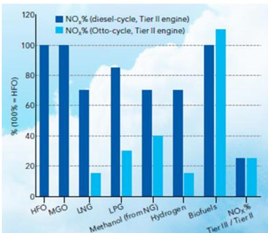
Figure 2.1 NO<sub>x</sub> emissions depending engine type, alternative fuels compared to HFO.
