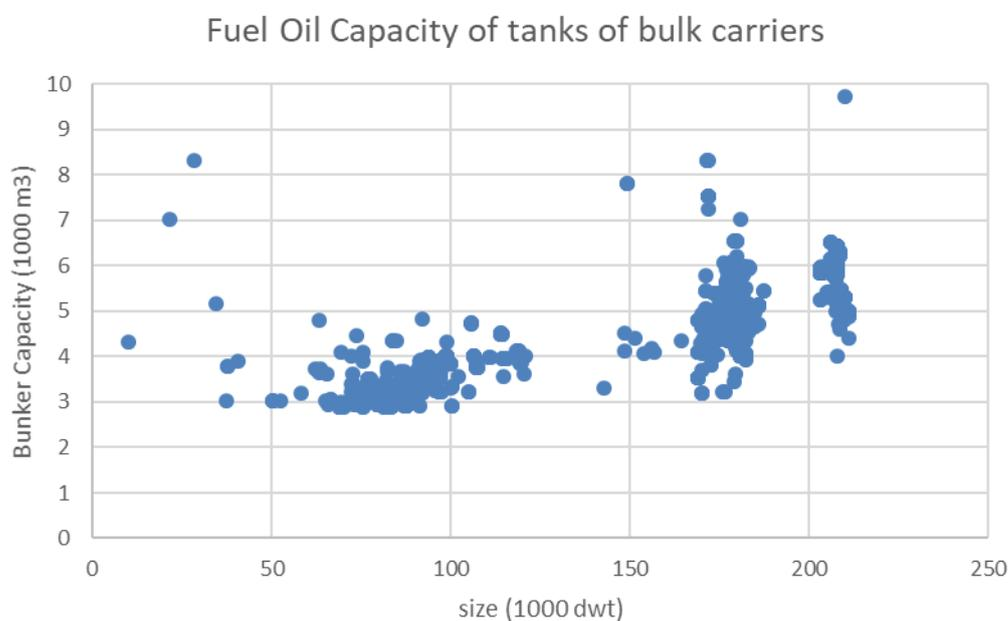
Figure 3.13 Bunker fuel tank size of bulk carriers
