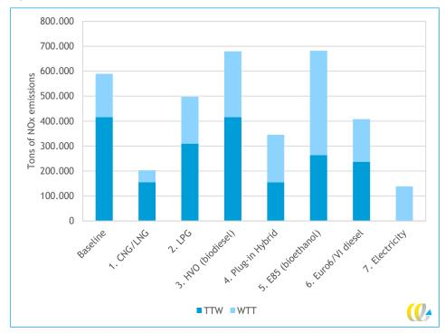
Figure 15 - Well-to-wheel NO<sub>x</sub> emissions in the different scenarios in the EU27
