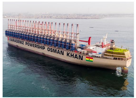
Figure 1 - An example of a self-propelled powership
