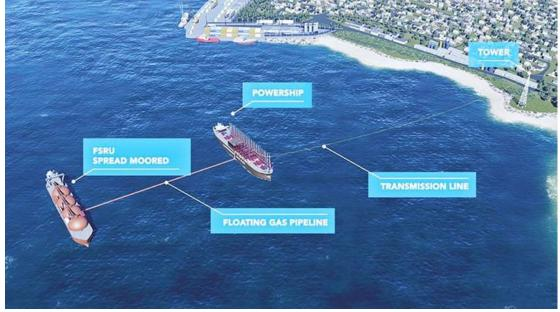
Figure 4 - Example of a 'power island', a combination of a floating powerplant and an FSRU
