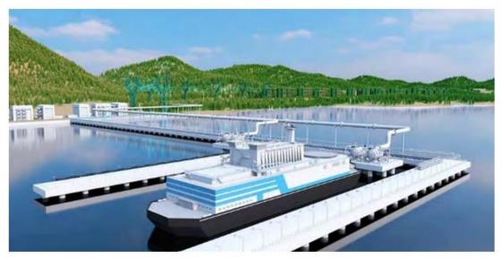
Figure 9 - Optimized Floating Power Unit with two RITM-200M rector plants
